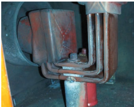
7. Glastic stand-offs used in many of the original cells were replaced with more durable Crown-sulators
